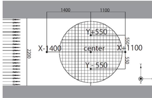
Figure. 2 Measurement points for approach flow velocity
