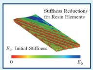
Legitimate damage models for carbon fiber and resin are obtained independently by simple material models.
