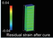
Initial defects arising in cure process are estimated for optimum temperature control.
