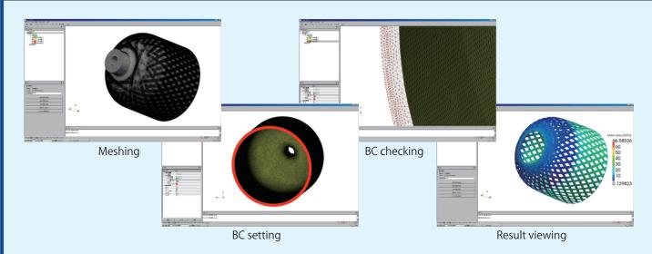
• Analysis and boundary condition settings for pre-processing and outputting BMP, output files for AVS, and FEMAP for post-processing are now available.
